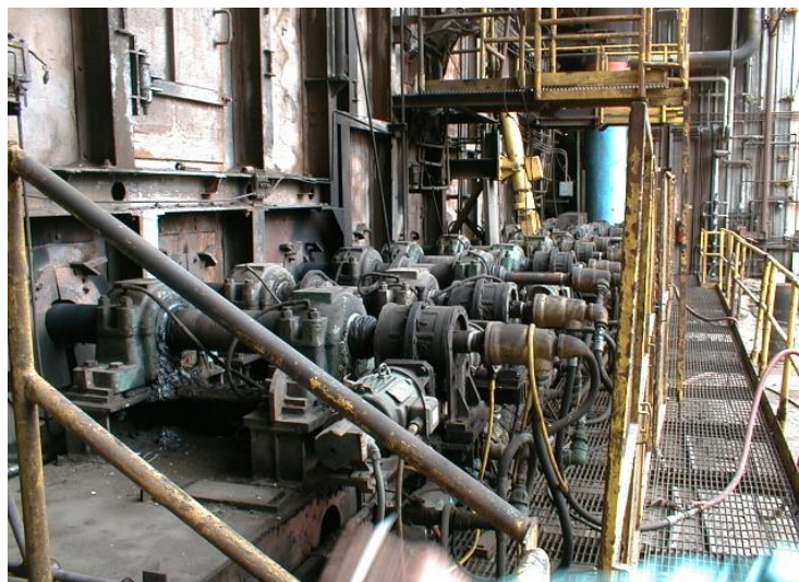
Figure 19: Old In-Furnace Charge Rolls
