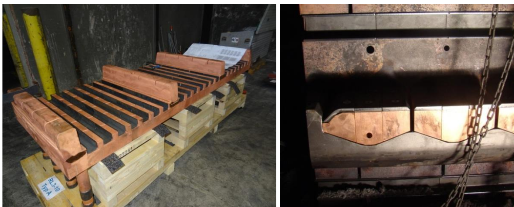
Figure 2.2 Staves with cooled ledges at workshop and ledge with patented exchangeable elements
