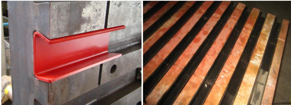
Figure 2.3 Staves with patented steel blades
