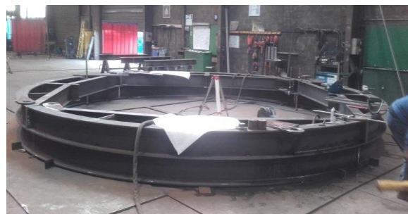
Figure 4.2 Patented Paul Wurth stave handling tool introduced through top cone
