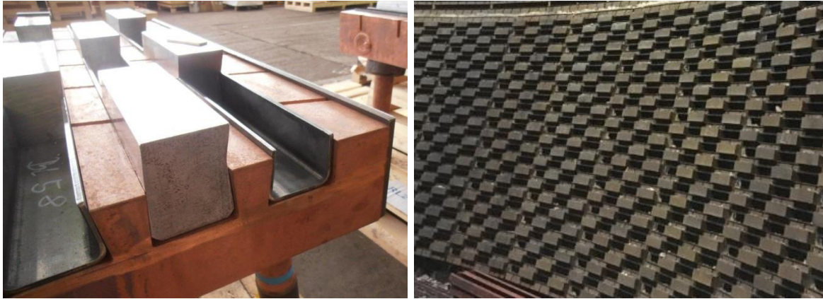
Figure 2.1 Staves with patented steel blades and steel inserts at workshop and during erection
