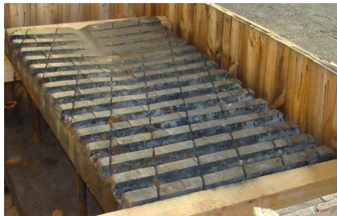
Figure 2.4 Damaged staves with the 2 typical wear patterns at the middle top and according to radius
