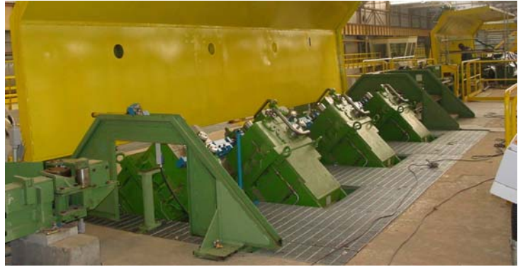
Figure 7 - The monoblocks consist of stands arranged at 90° to each other and 45° to the horizontal line, with an alternate left- and right-hand configuration. This configuration together with the symmetric roll gap adjustment provides a no-twist and fixed pass line operation.
