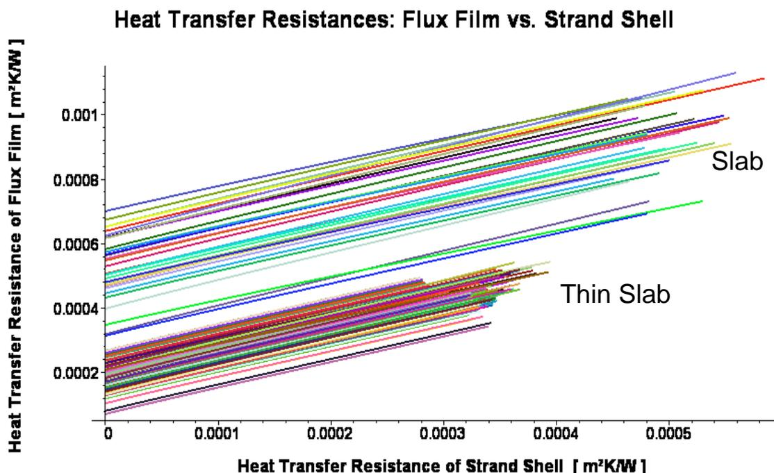
**Figure 8:** Linear relation between the heat transfer resistance of the slag film and the heat transfer resistance of the strand shell, 300 caster data sets .
