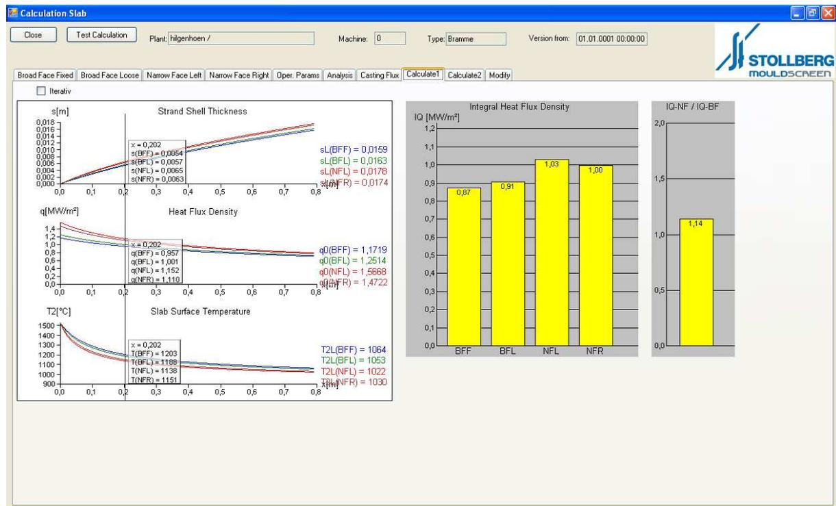
Figure 3: Strand shell thickness, heat flux density and slab surface temperature.
