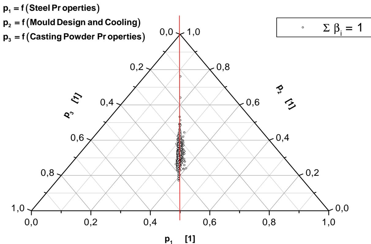
**Figure 9:** Ternary diagram of the three non-dimensional meniscus parameters  $p_1$ ,  $p_2$  and  $p_3$ , about 1000 caster data sets.
