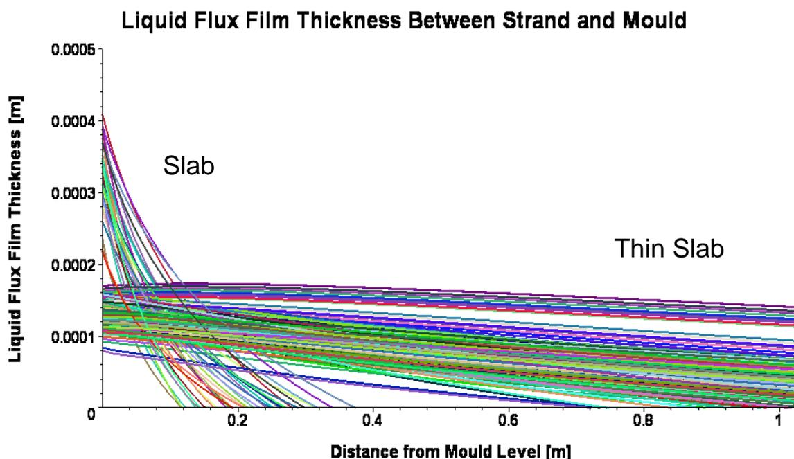
**Figure 7:** Liquid slag film thickness from mould level to mould exit of slab- and thin slab-casters, 300 caster data sets.
