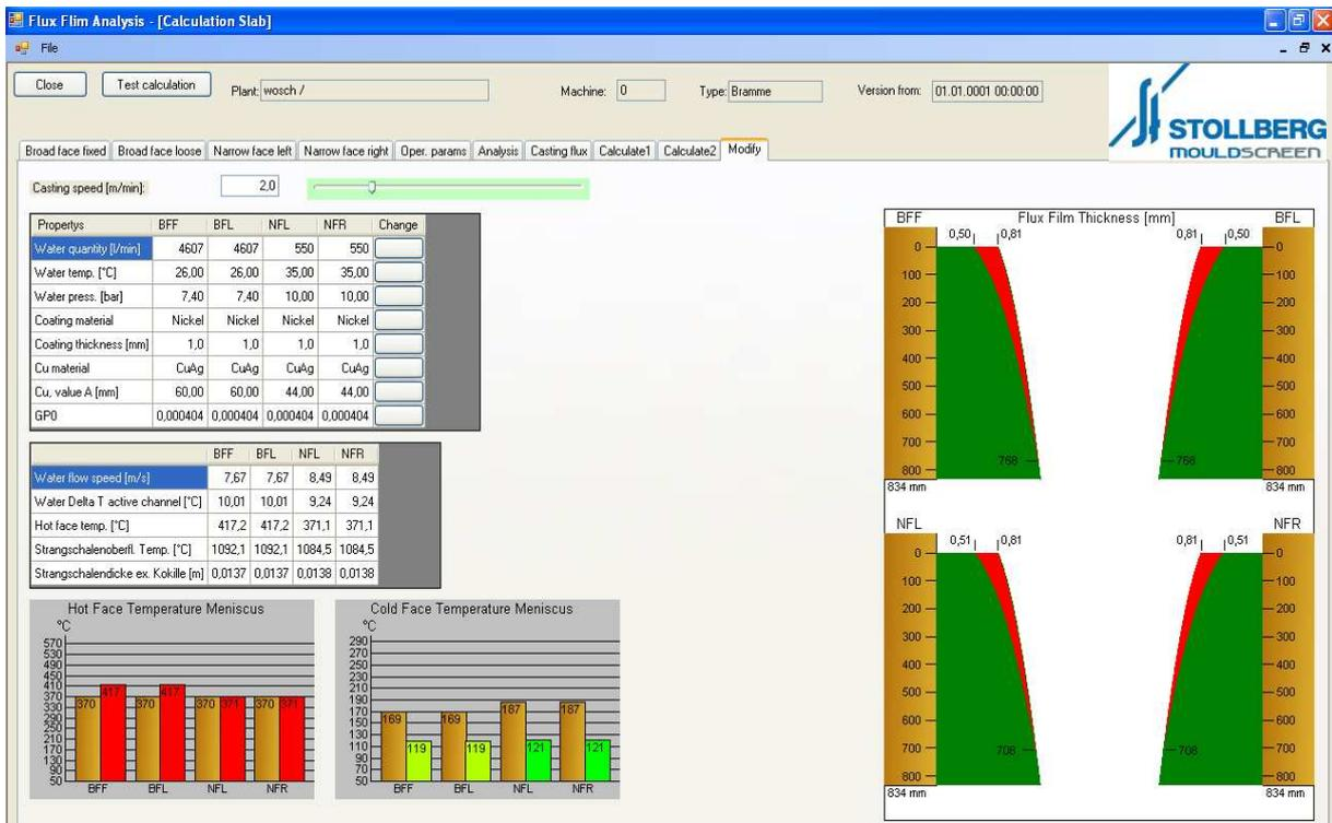
**Figure 6:** Modify tool: variation of operation parameters and its influence on copper plate temperatures and liquid/solid slag film thickness (red/green), e.g. Casting speed: 0.8 m/min (5 a) → 2.0 m/min (5 b).
