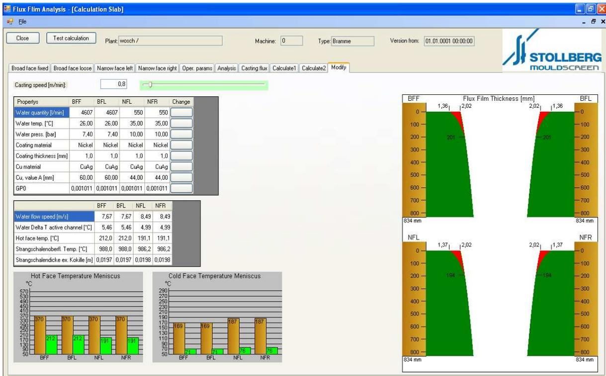
**Figure 5:** Modify tool: variation of operation parameters and its influence on copper plate temperatures and liquid/solid slag film thickness (red/green), e.g. Casting speed: 0.8 m/min (5 a) → 2.0 m/min (5 b)
