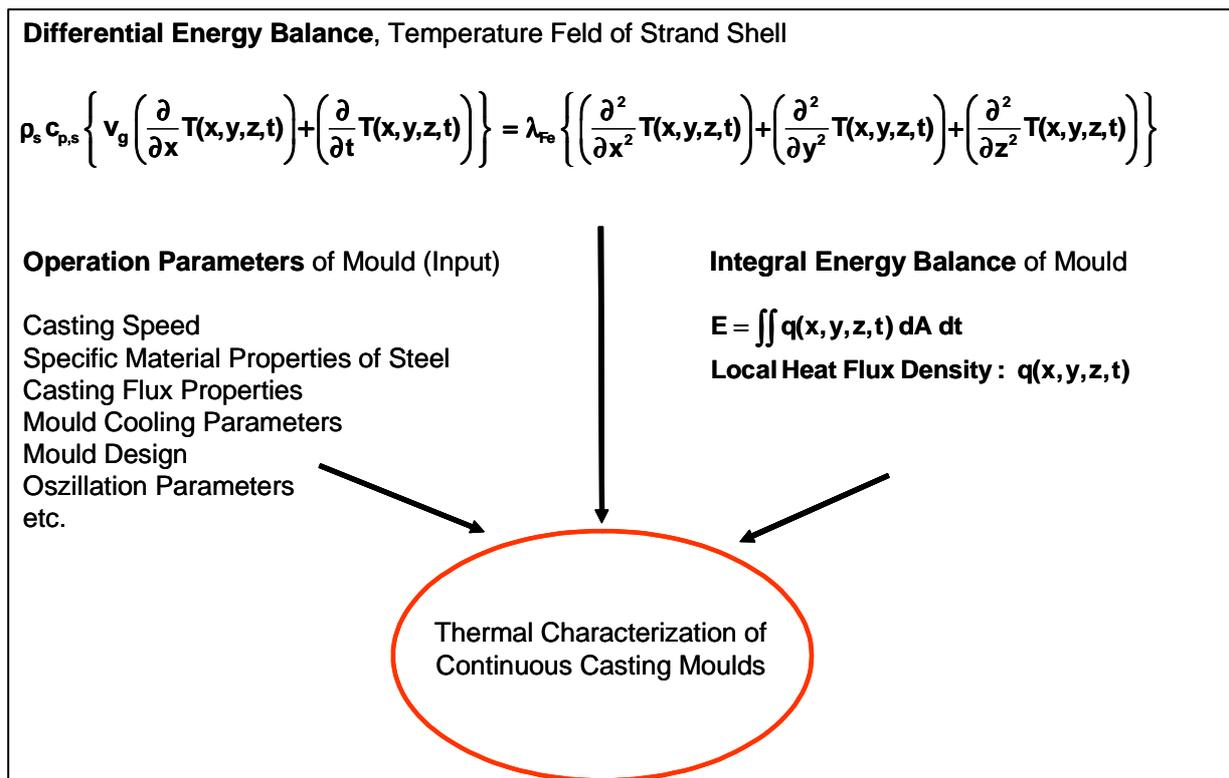
**Figure 1:** Basic principles and model components.
