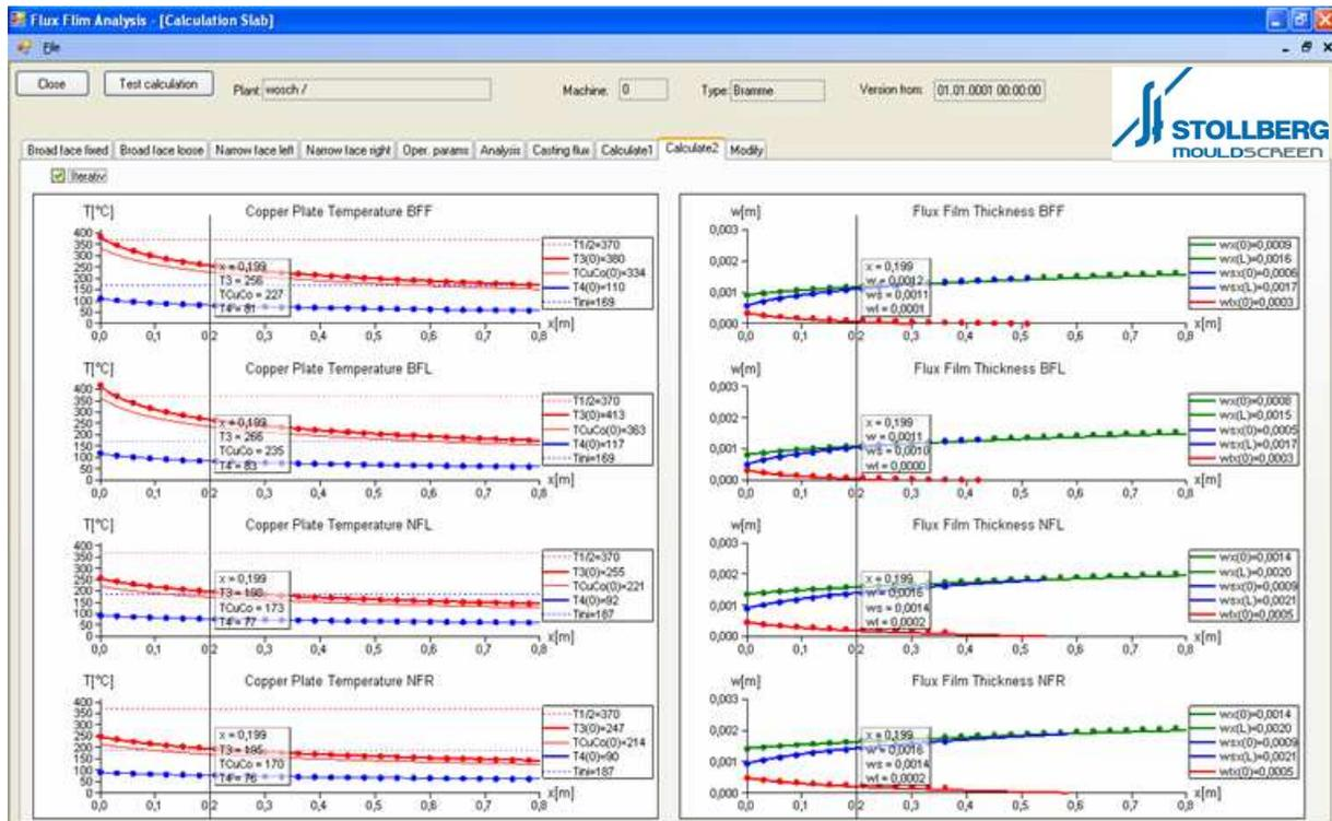
Figure 4: Copper plate temperatures and slag film thickness.
