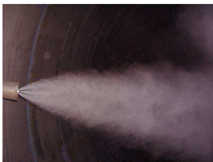
Figure 13: Dual flow water mist
