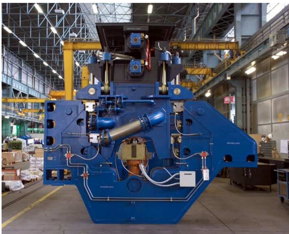
Figure 6: Mould and its oscillating, width adjustment devices.
