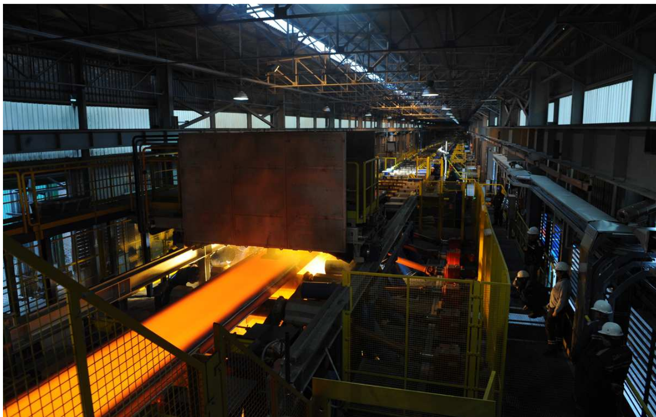
Figure 9: Slab during first casts
