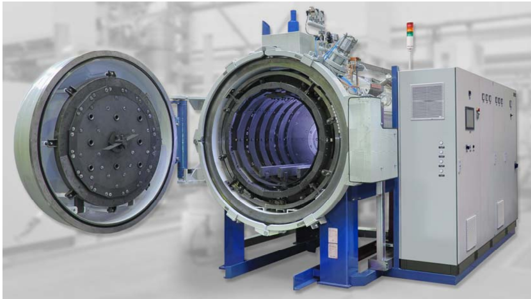
Fig. 2. Seco/Warwick 15.0VPT-4035/36IQCN vacuum furnace (Vector - vacuum furnace line). The parts under study made from Pyrowear® Alloy 53 steel were placed, together with a ballast charge of approx. 250 kg (551 lb), which reflected the standard conditions of industrial processes.
