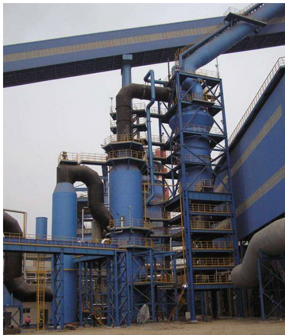
Fig 8: BF gas cleaning plant (axial cyclone, AG scrubber, mist eliminator of BF2, Tianjin, PR of China).
