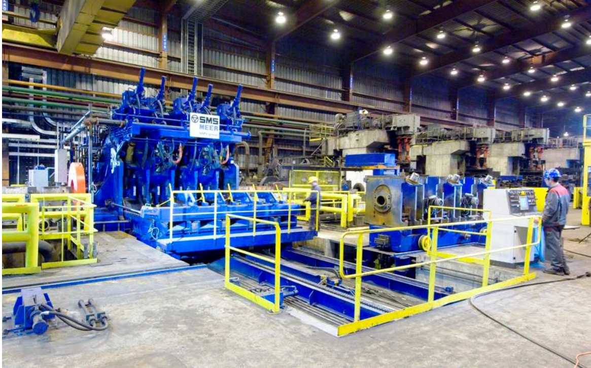
Figure 4. The PSM during stand change. In foreground the changing car, on the right the new mill set-up ready to be transferred on-line.
