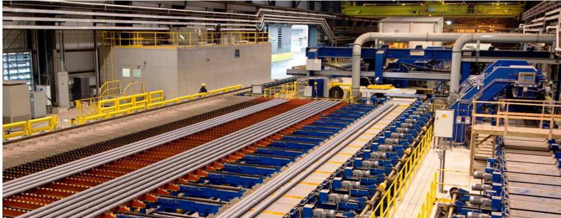
Figure 8: Cooling bed exit with cut-to-length saws
