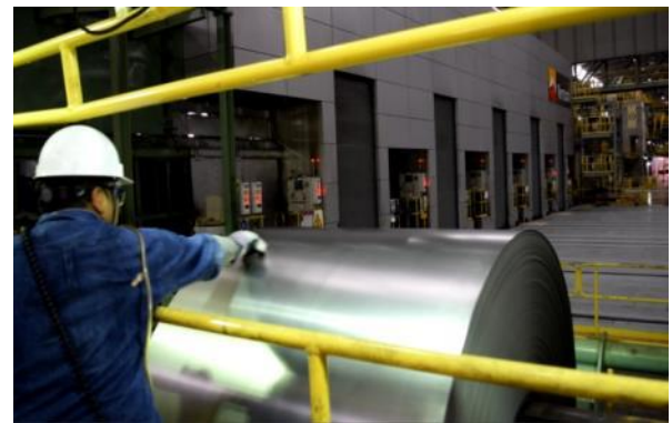
Figure 15. Operator stoning the top side to reveal defects.
