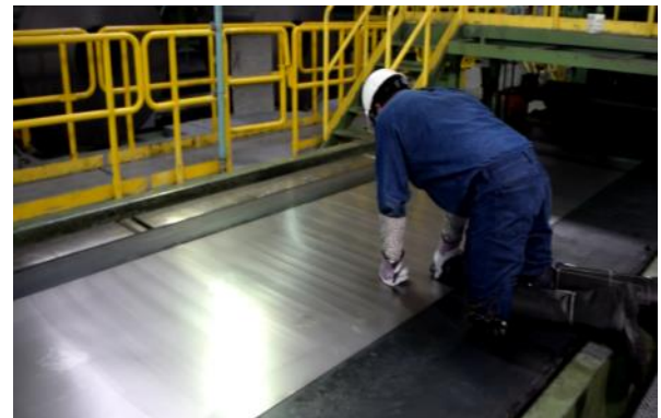
Figure 14. Operator stoning the bottom side to reveal defects very important practice to evaluate superficial quality for automotive market.
