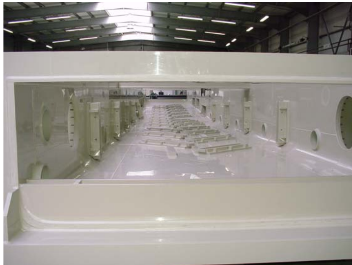
Figure 2. Pickling tank 26m long
