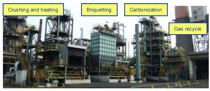
Fig.9 Overview of a pilot plant of 30t/d for the ferro-coke production
