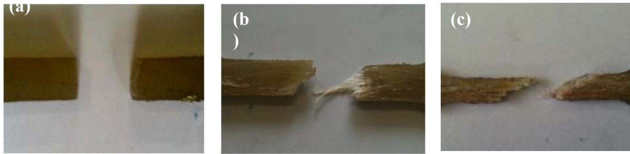
Figure 6. Fracture tip of tensile-ruptured polyester composites with (a) 0%, (b) 20% and (c) 40% of volume fraction of thinner curaua fibers.
