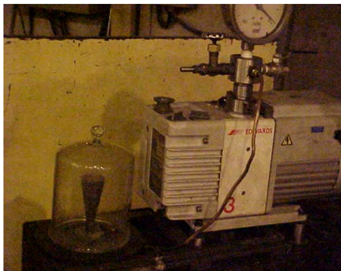
Figure 6. Vacuum pump during the test solidification at reduced pressure.
