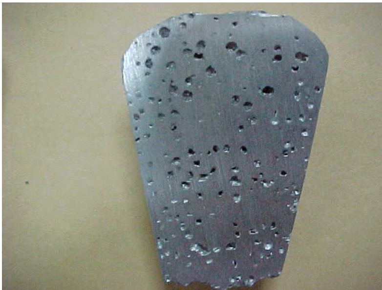
Figure 9. Appearance of the specimen - liquid metal density: 2.58 g/c.c.
