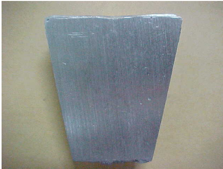
Figure 8. Appearance of the specimen - liquid metal density: 2.70 g/c.c.
