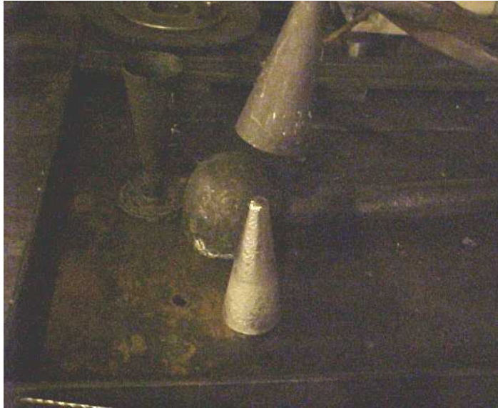
Figure 7. Extraction of the test piece from the mold after solidification of the sample.
