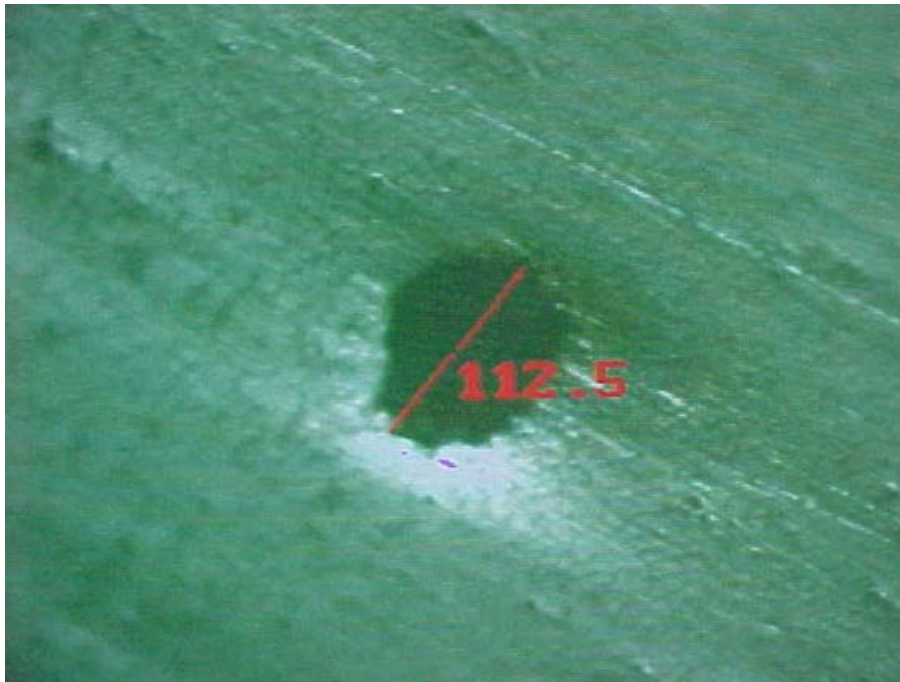
Figure 14. Pore diameter of 112.5 microns (0.1125 mm) observed with the optical microscope Olympus 100X.
