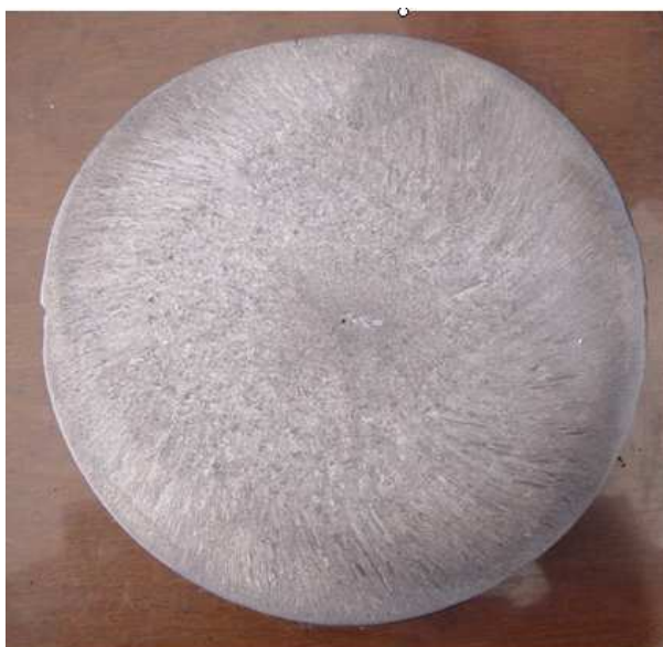
Figure 7: Macro etch of T91 stainless steel, casting speed 1.20 m/min.
