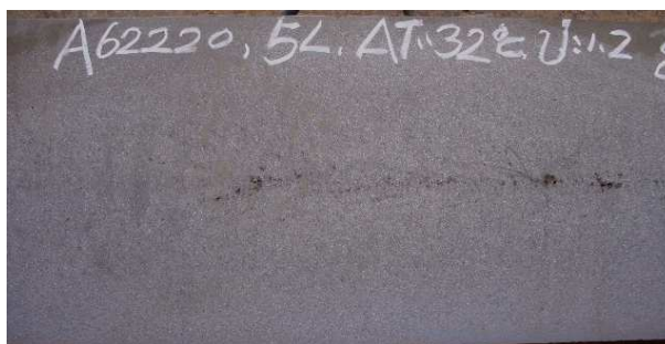
Figure 11: Longitudinal sample with SIMETAL DynaGap Soft Reduction ® .
