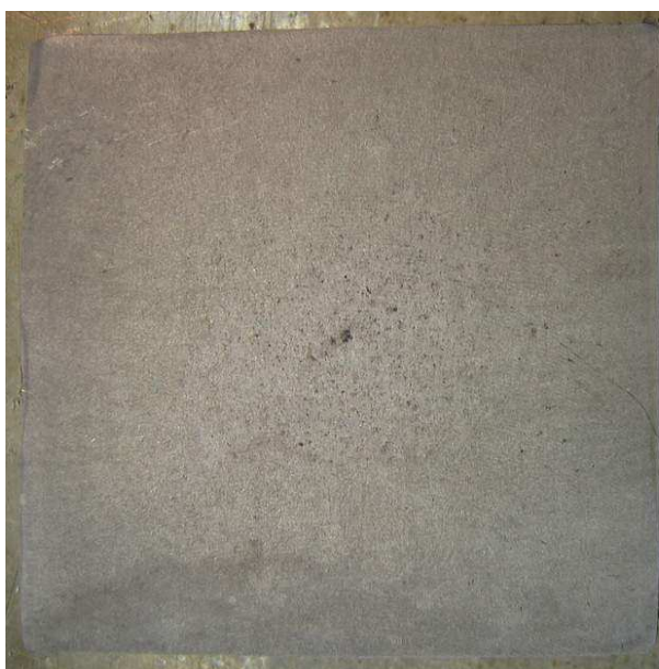
Figure 2: Heat N. 15564, macro etch of 35GS, casting speed 6.6 m/min.
