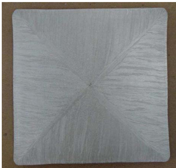
Figure 5: Macro etch of 316 Stainless steel, casting speed 1.6 m/min.
