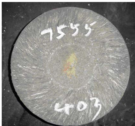
Figure 8: Macro etch of SUP13CRr stainless steel, casting speed 1.20 m/min.
