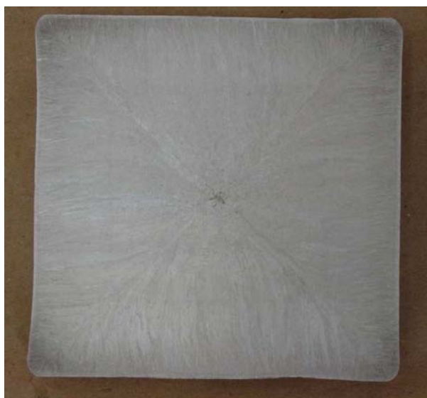
Figure 4: Macro etch of 304 Stainless steel, casting speed 1.6 m/min.
