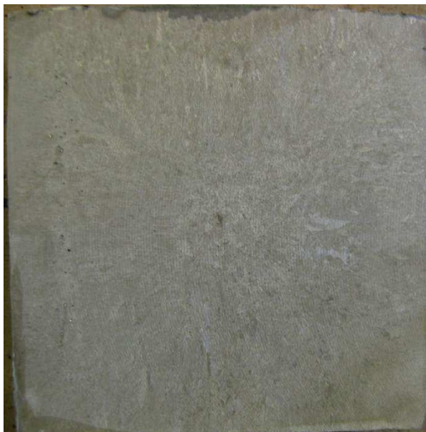
Figure 1: Heat N. 64083, macro etch of StSp3, casting speed 7.1 m/min.
