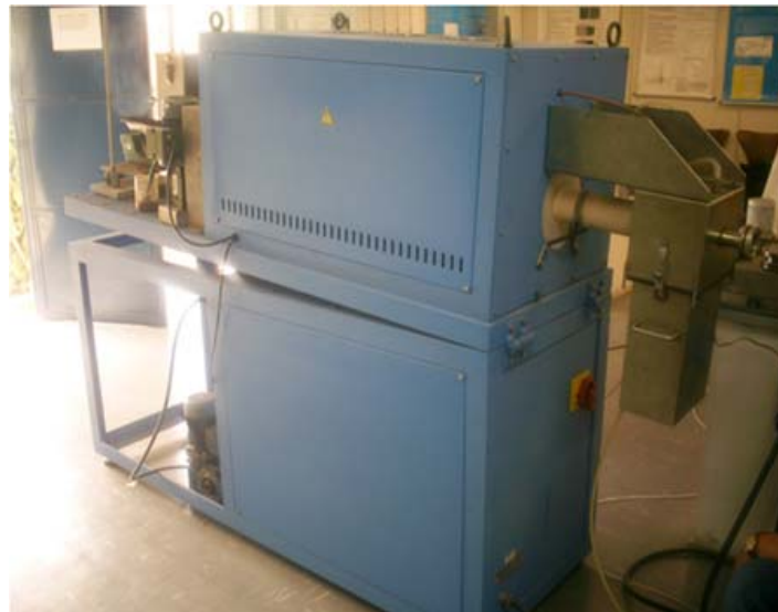
Figure 2. System used for the experiments (laboratory rotary kiln furnace, electrically heated).
