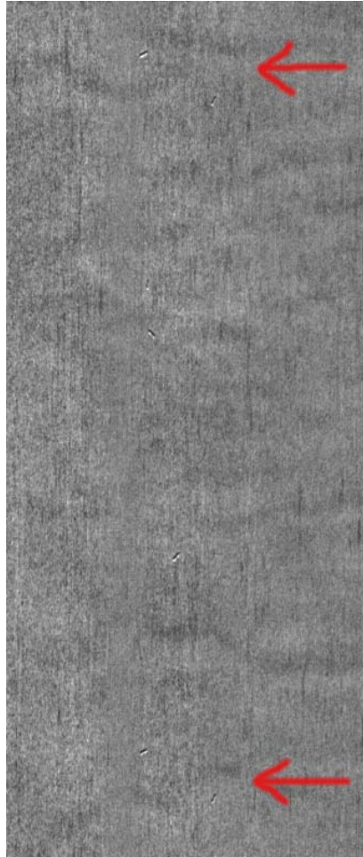
Figure 4b. Another picture of the same 2.2 m picture that is 0.4 m long in rolling direction. The same roll mark is now visible twice.
