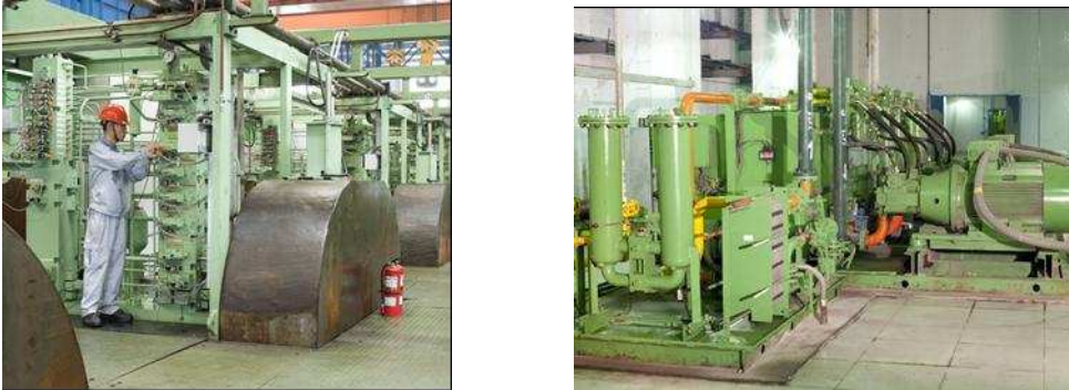
Figure 6: hydraulic systems in modular design
