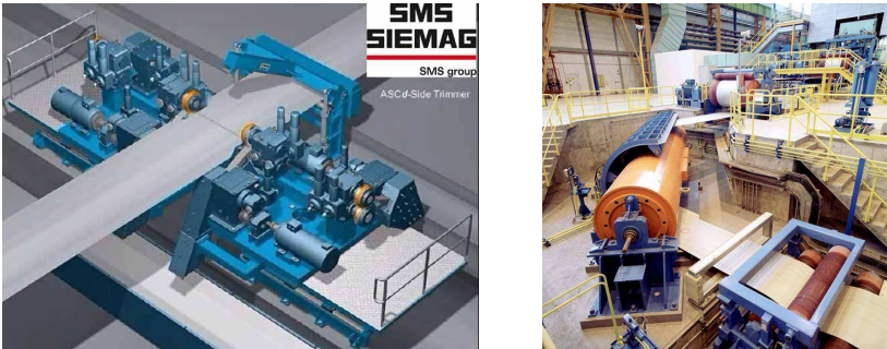
Figure 12: ASD Side trimmer (l), twist roll in the entry section of a PL/TCM (r)
