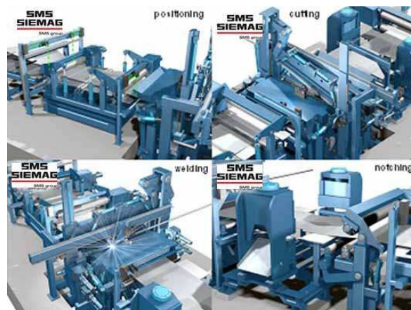
Figure 11: Welding cycle of the new welding machine
