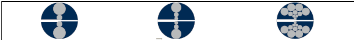
Figure 1: Rolling mill classification 4-hi / 6-hi / 20-hi
