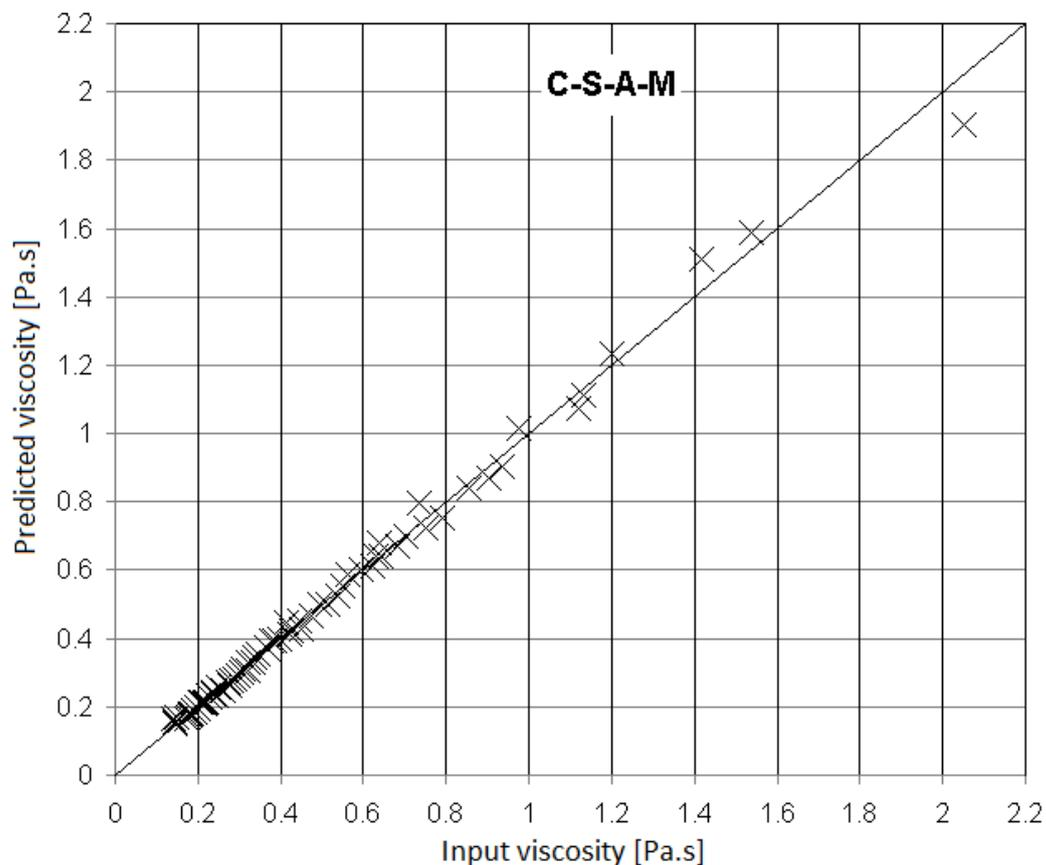
**Figure 2.** Predicted viscosity values as a function of the input values, C-S-A-M system
