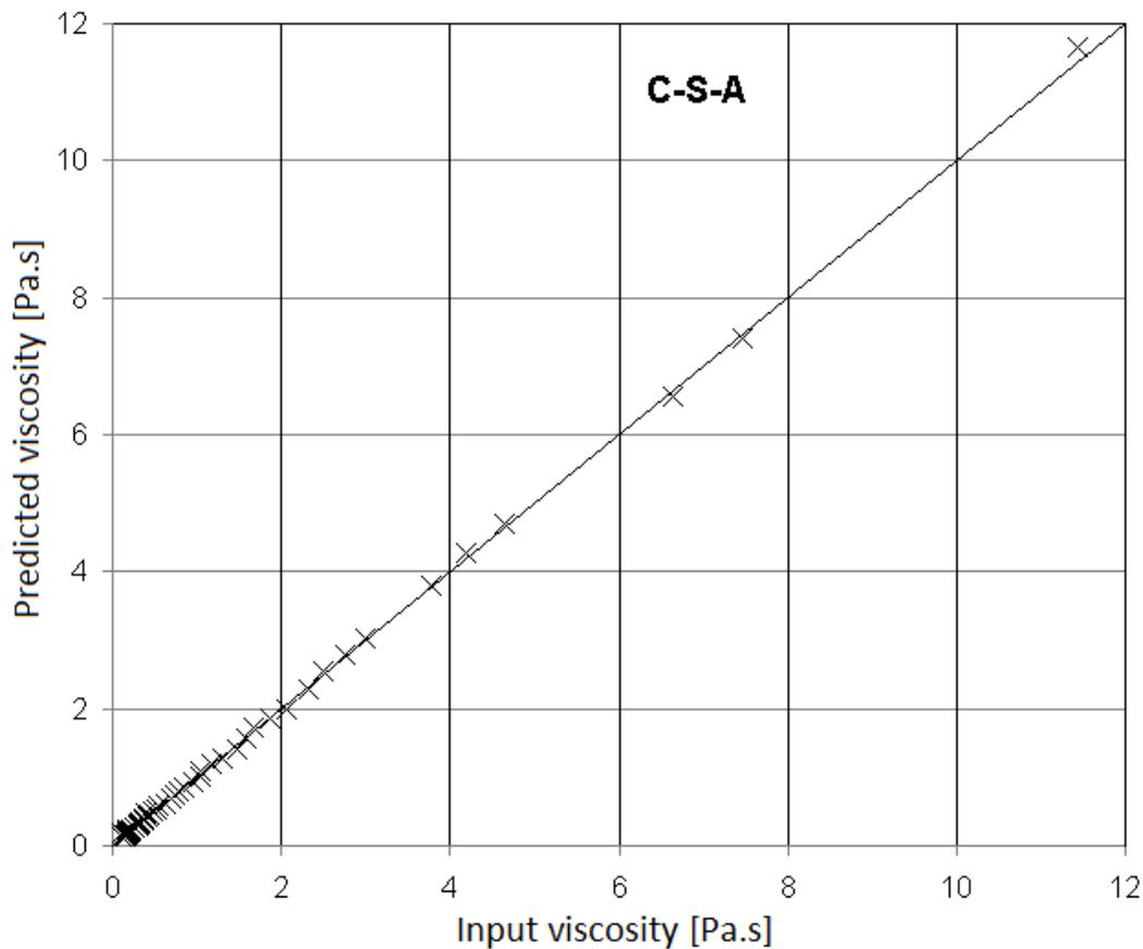
**Figure 1.** Predicted viscosity values as a function of the input values, C-S-A system
