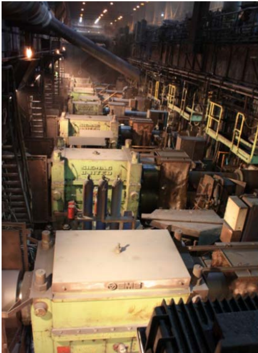
Figure 6. Drive side of finishing mill.
