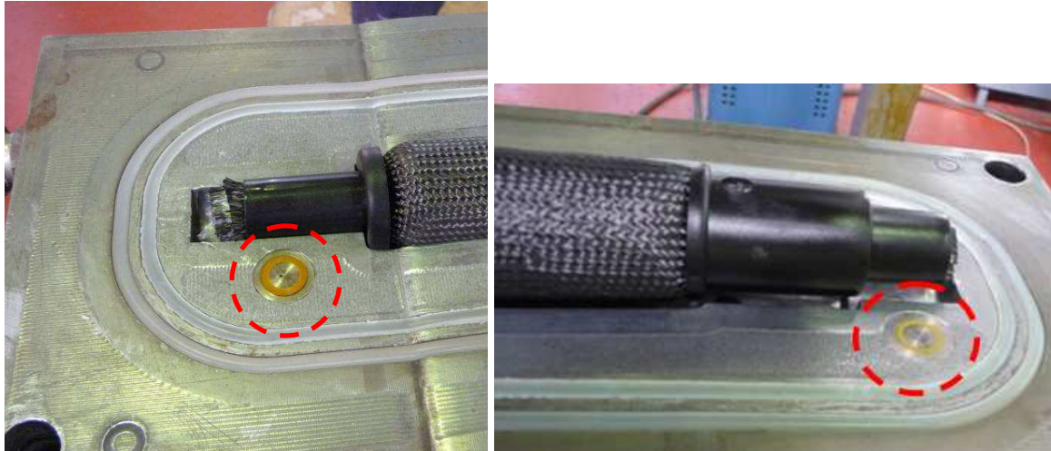
Fig.5. Flash mounted sensor at the cavity's margin near the inlet (left) and outlet (right) gates.
