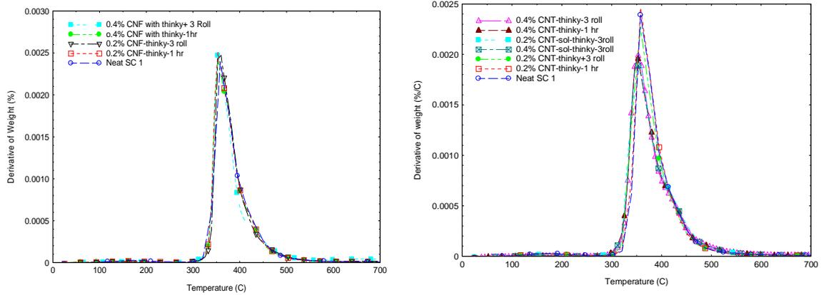
Fig. 6. Derivative of weight vs. temperature curve for MWCNT/epoxy & CNF/epoxy.
