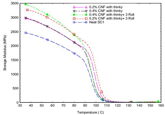
which affects the overall mechanical properties. It can be observed from Table 2 that 0.2 wt% CNF with thinky+ 3roll mixing showed best strength, modulus and maximum strain values compared to all sets of data.
