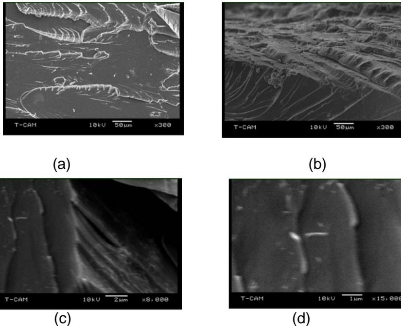
Fig.8. Micrograph of 0.4wt% MWCNT infused epoxy with thinky+ 3Roll mixing at higher magnification.
