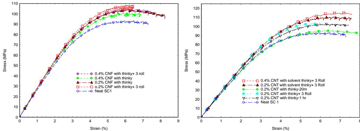
Fig.2: Stress- strain curves of epoxy and CNF/epoxy (left) and MWCNT/epoxy (right).
