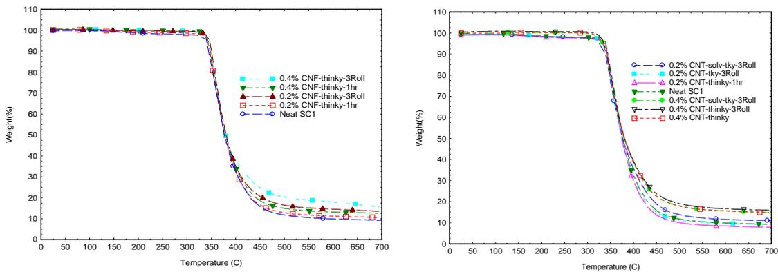
Fig.5: Weight (%) vs. temperature curves of epoxy and MWCNT/epoxy (left) and CNF/epoxy.
