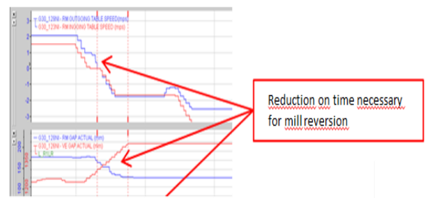
Figure 11. Roughing Mill reversion before total mill gap positioning.
