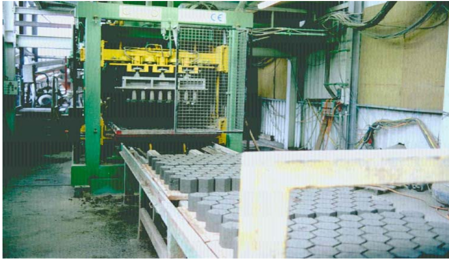
Figure 4: Brick making machine with punches lifted above the moulds. Green bricks are pushed forward on their wooden pallets about every 20 seconds.
