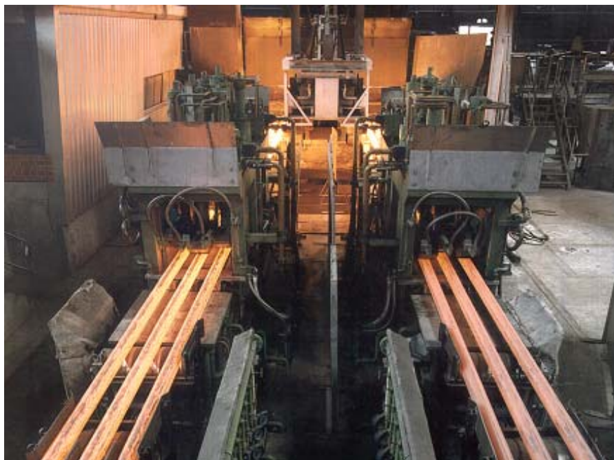
Figure 10: Horizontal continuous caster for mini mills
