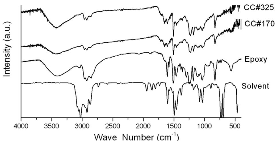
**Figure 3:** FTIR spectra of the CACMs compared with the epoxy resin and the solvent spectra.
