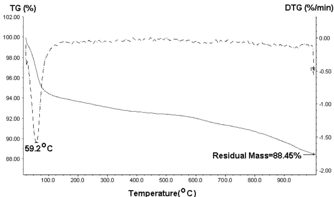
**Figure 1:** The TGA curve and its derivative showing the thermal decomposition temperature and the residual mass of as received activated carbon (CR-micro).
