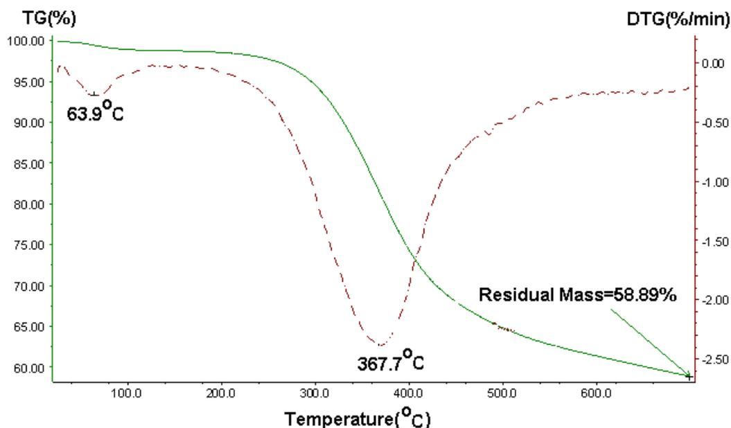
**Figure 2:** The TGA curve and its derivative of CACM (CC-CR) showing the thermal decomposition temperatures and the residual mass of its constituents.
