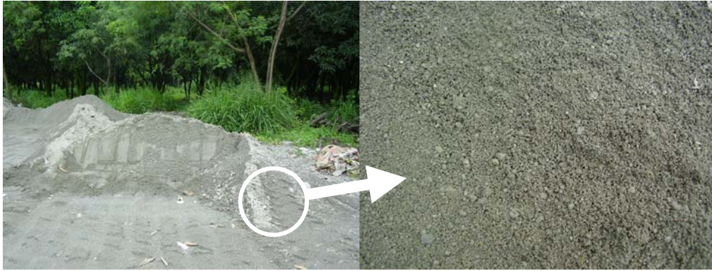
Figure 1 – Non-metallic fraction of steel slag (0-4mm)
