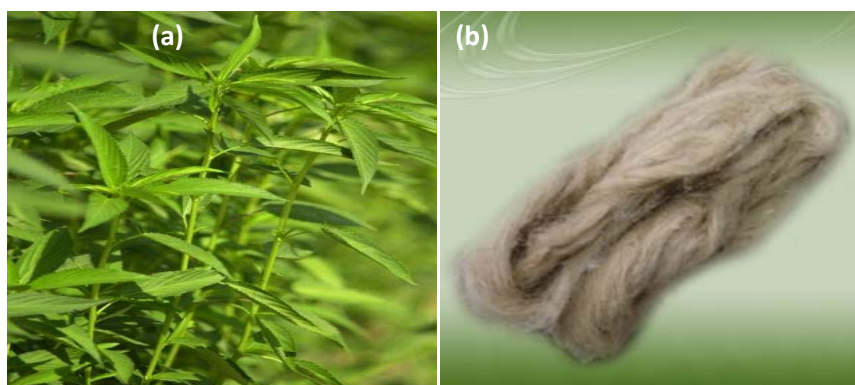
Figure. 1. (a) Typical aspect of jute; (b) bundle of jute fibers used in this investigation.
