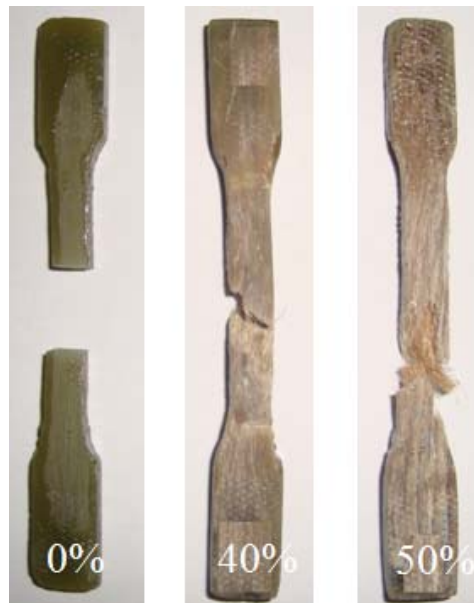
Figure 3. Tensile ruptured specimens for each volume fraction of jute fiber incorporated into the epoxy matrix.
