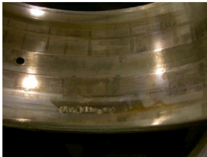
Figure 2. Showing wear, corrosion and spalling in bearing raceway
