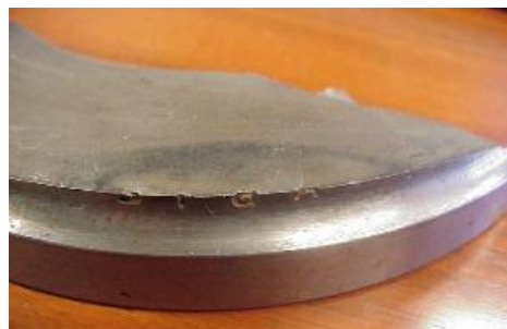
Figure 2. Tungsten carbide roll breakage with EDM marking.
