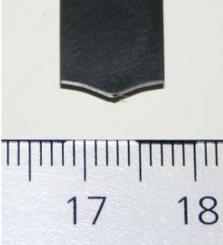
Figure 13. Notching tool for chamfered concentric rebar
