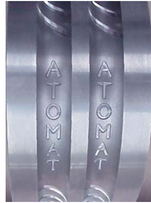
Figure 5. Mark on 16mm rebar, 8-inch tungsten carbide roll
