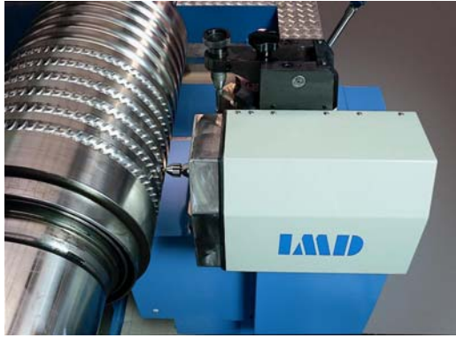
Figure 4. Integrated marking device (IMD).
