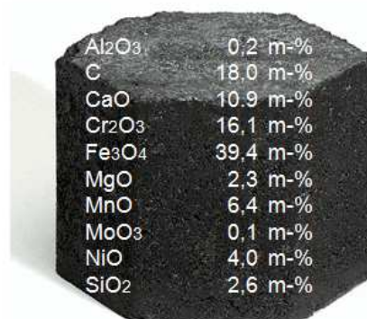
Figure 3 - Self-reducing test brick.
