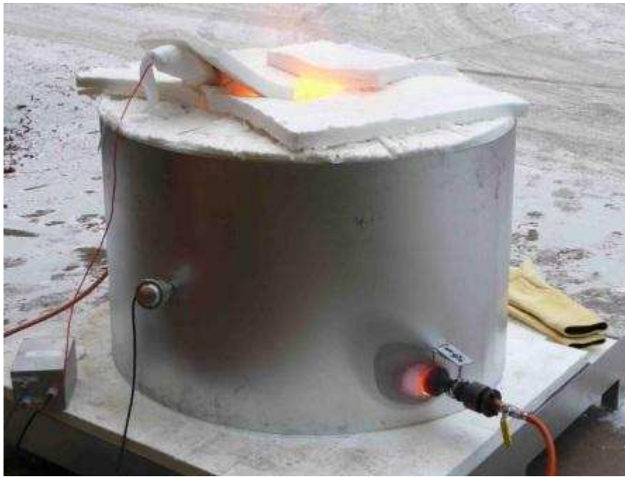
Figure 6 - Gas fired test furnace for smelt-reduction trials.
