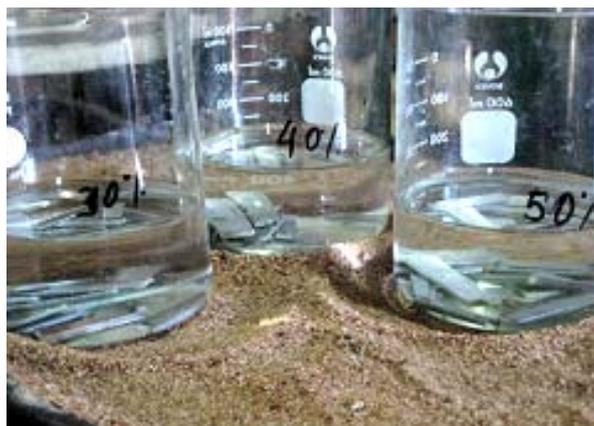
**Figure 7.** Residues after pure HCl attack.
