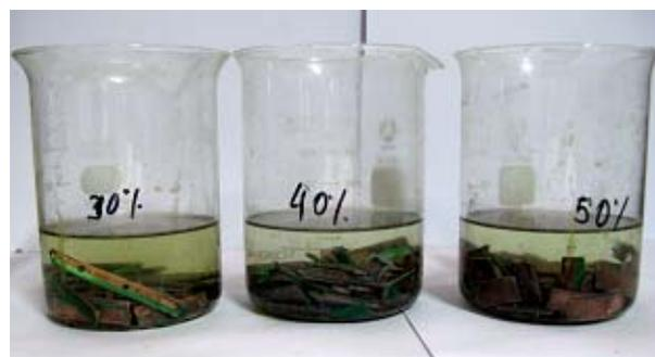
Figure 11. Solutions after  $\text{Cu}^{2+}$  cementation
