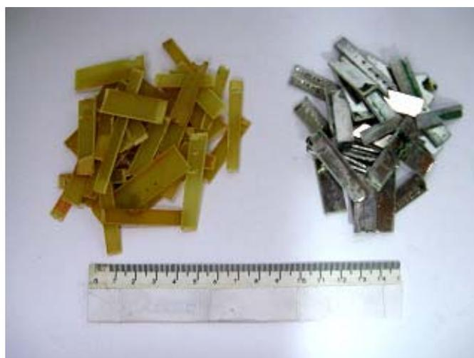
**Figure 9.** PCB chips before and after stripping process.
