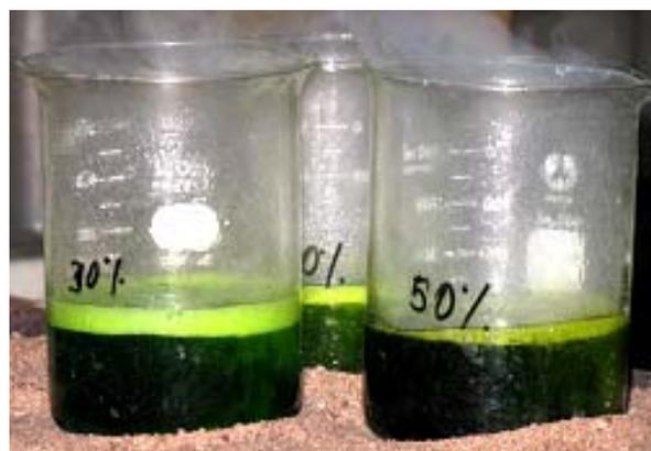
**Figure 8.** Residues after HCl + HNO<sub>3</sub> attack.
