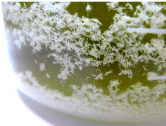
**Figure 13.** Lead chloride precipitate
