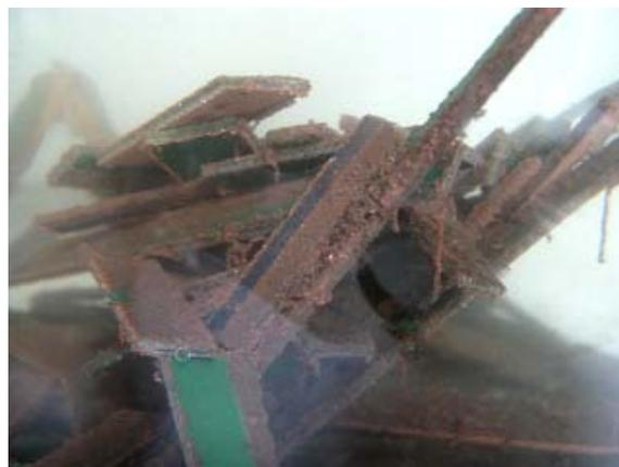
Figure 12. Appearance of cemented copper .
