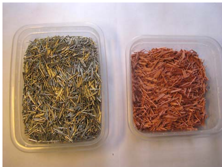
Figure 6. Visual appearance of the waste before tin recovery process (left) and after tin removal (right), with the typical color of copper.
