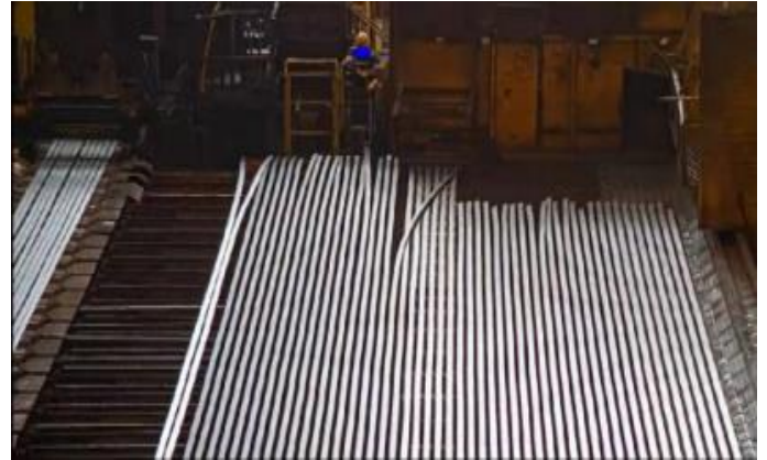
Figure 4 Warped bars in the cooling bed
