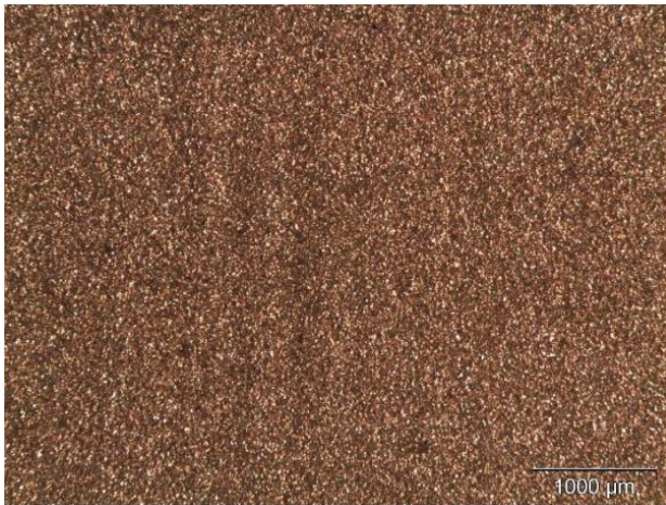
Figure 9 Etched straight sample. 2,5x zoom.
