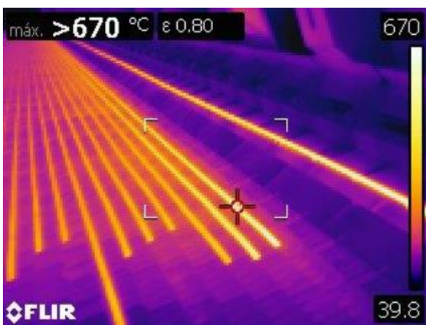
Figure 3. Temperature of the bars arriving the cooling bed.
