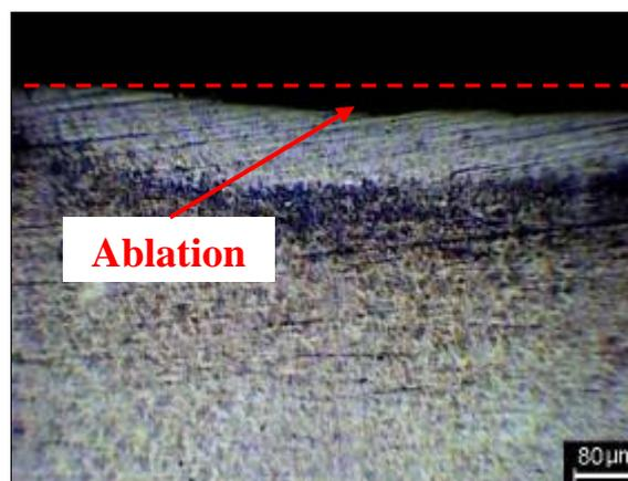
**Figure 4:** Transversal section of the laser treated zone (with ablation) and the base of the material, 2% Picral reagent.
