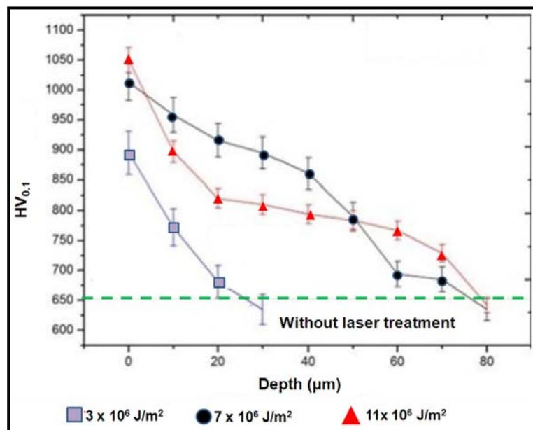
**Figure 6:** Profile obtained from Vickers microindentation of the laser treated zones using different energy intensities.
