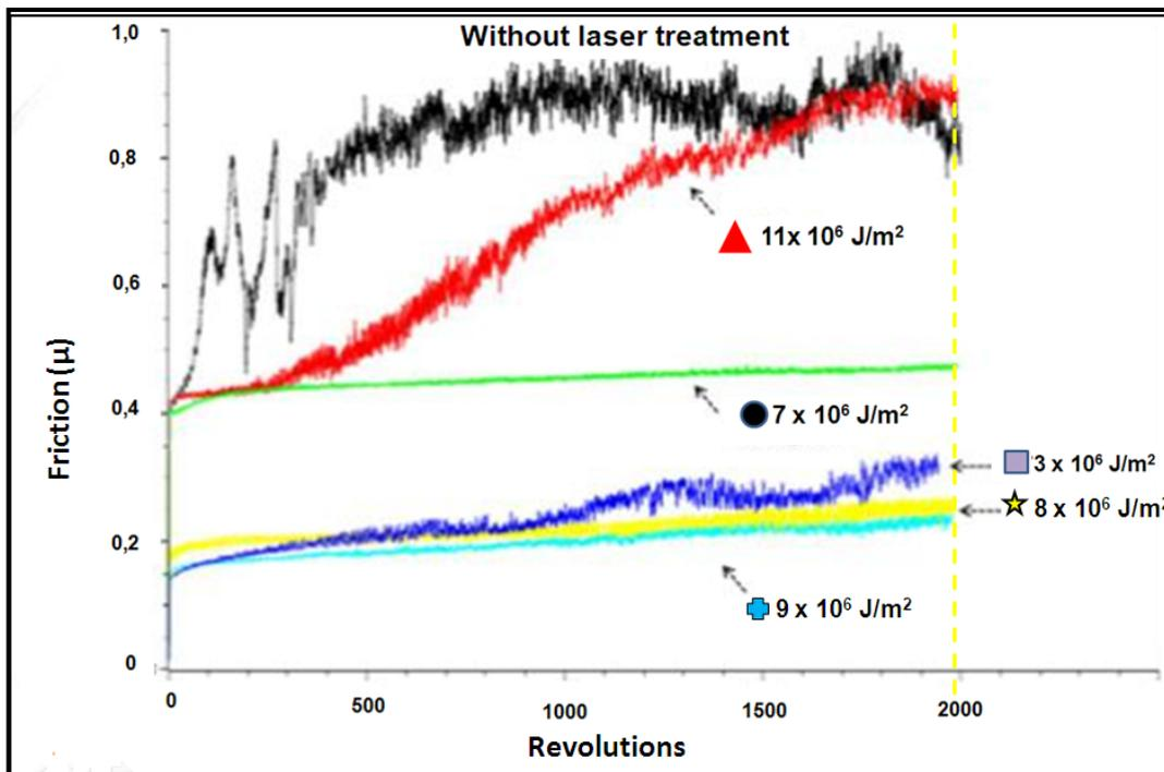
**Figure 10:** Friction coefficient for the laser treated pairs.
