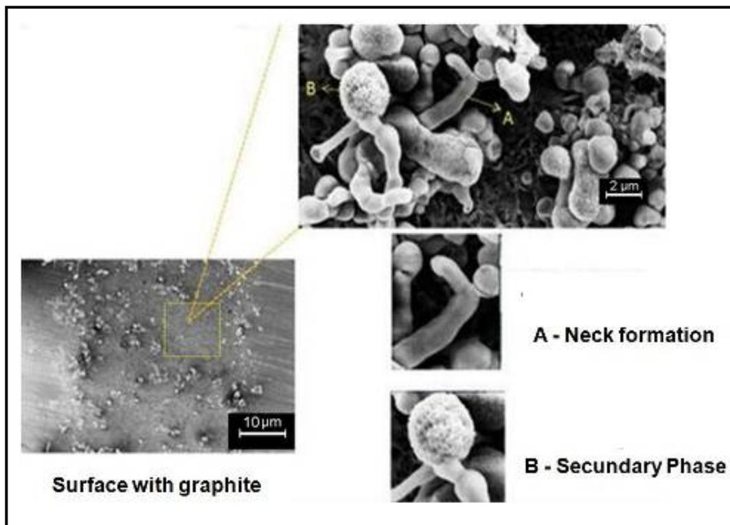
**Figure 7:** Morphology of the graphite coating fixed with an energy intensity of  $7 \times 10^6 \text{ J/m}^2$ .
