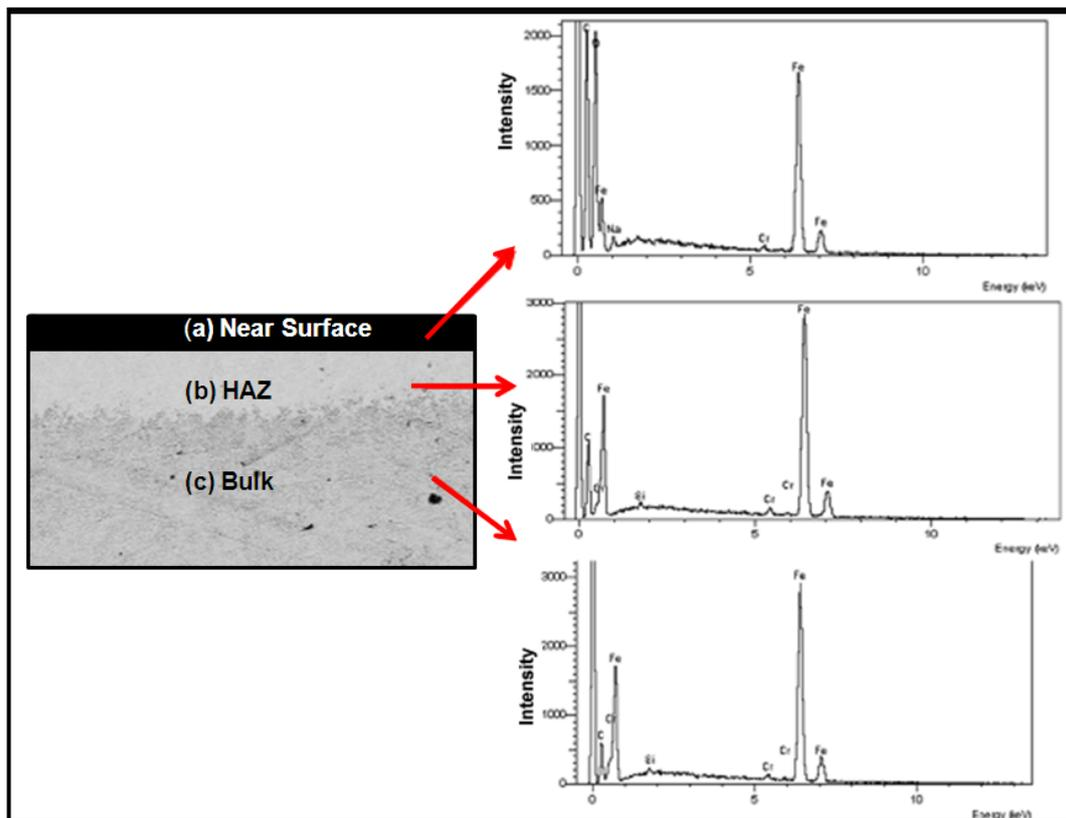
**Figure 8:** Chemical analysis of the transversal profile of laser treated AISI 52100 steel.
