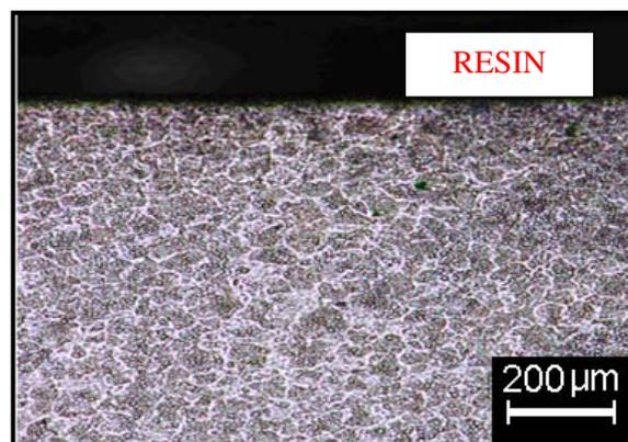
**Figure 2:** Microstructure of AISI 52100 steel, consisting of two distinct stages.
