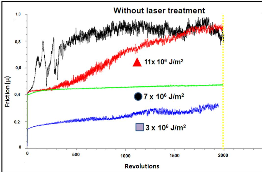
**Figure 9:** Results for the friction coefficients of samples with and without laser treatment.
