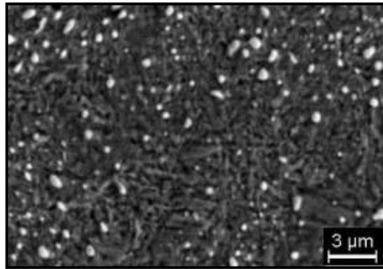
**Figure 3:** SEM of AISI 52100 steel, consisting of two distinct stages.
