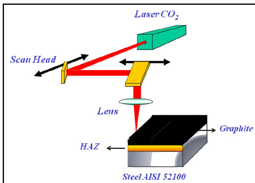
Figure 1: Schematic of AISI 52100 steel laser processing.
