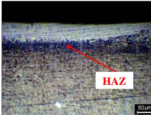
**Figure 5:** Transversal section of the laser treated zone (without ablation) and the base of the material, 2% Picral reagent.
