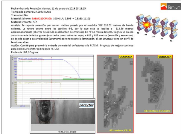
Figure 3. Example of detailed analysis of a substrate defect break.
