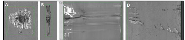
Figure 10: Images of critical surface defects (A transport abrasion, B scab, C Cross bending, D Strong scratch).
