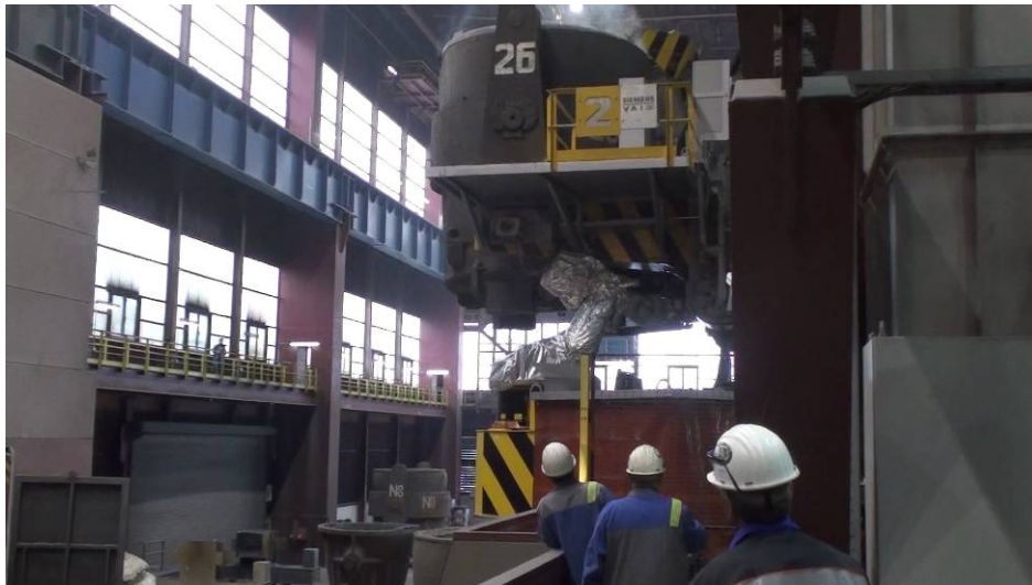
Figure 12. LiquiRob attaches the ladle shroud handling device on the first heat.
