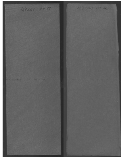
Figure 9. Macro etches centre segregation; position: middle; material: C75, C = 0.75%C.
