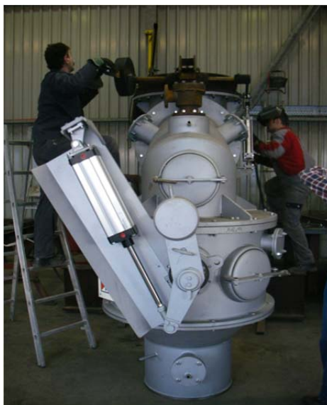
Figure 3. Sopreco ® Version 2 ready for installation on Coke Battery No.2.
