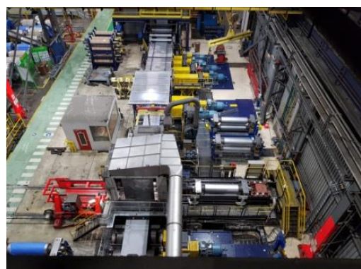
Figure 10c : Top view of skin pass and motorization completely dismantled
