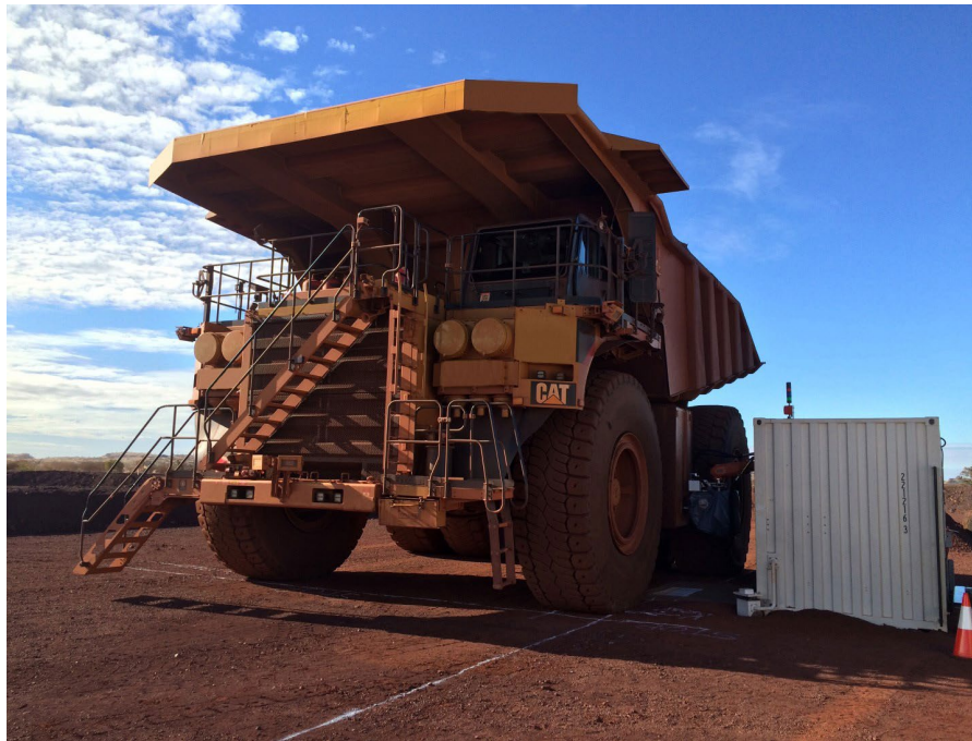
Figure 5. Robofuel on-circuit refueling of a CAT 793F. Iron Ore Site, Australia
