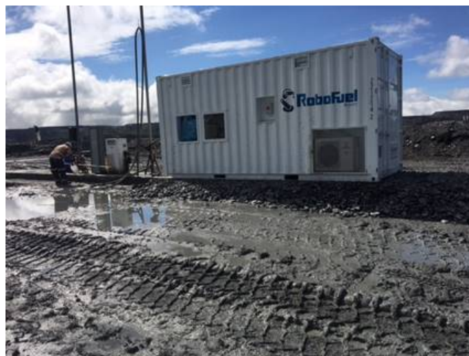
Figure 6. Robofuel retrofit to existing refuel bay. CAT 789D/E fleet, New Zealand
