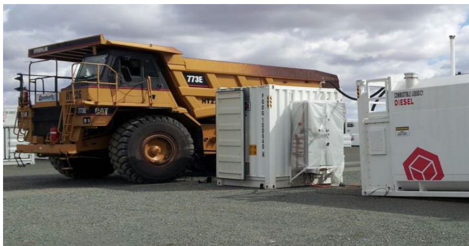
Figure 4. Robofuel prototype – refueling a CAT 773E.Parkes, Australia
