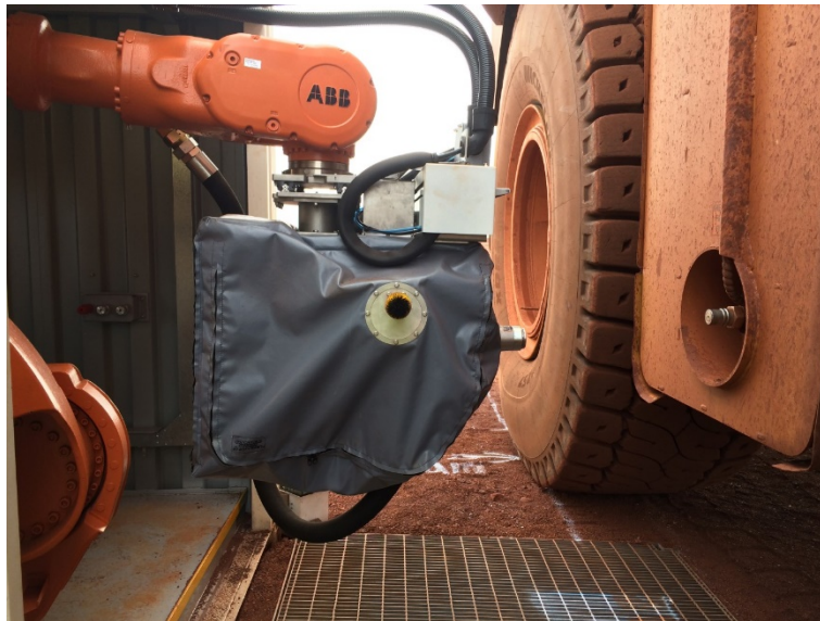
Figure 2. Robofuel refueling a CAT 793F vehicle, on-circuit. Iron Ore Site, Australia
