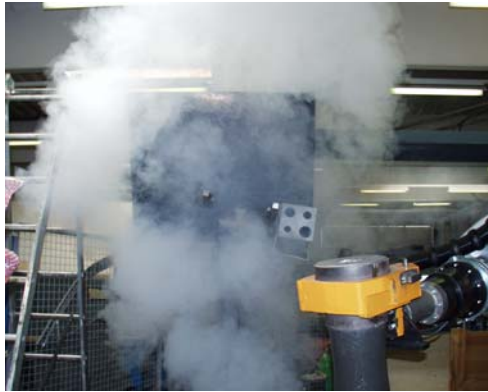
Figure 5 Position detection tests under steel plant conditions
