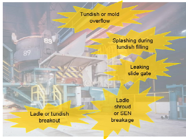
Figure 1 Dangers on casting platform
