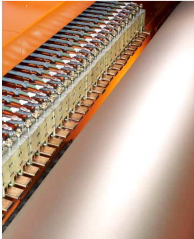
Figure 3. An Example for the homogeneous surface of a textured roll and also the arrangement of the electrode heads with the copper made electrodes, source: WaldrichSiegen.
