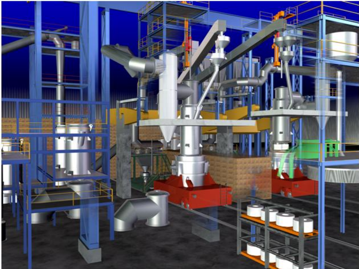
Figure 7. Schematic of the Duplex Vessel RH unit at NLMK.
