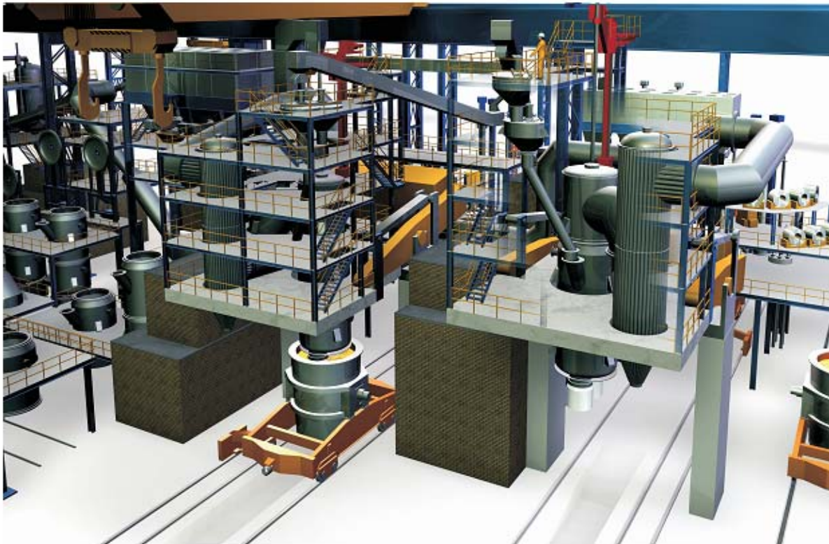
Figure 5. Schematic of the Duplex Vessel RH unit at MMK.
