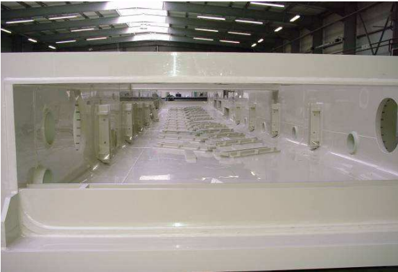
Figure 4: Cross section of pickling tank
