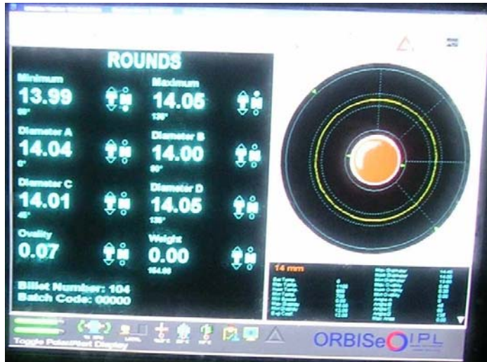
Figure 11. Shijiazhuang Round dia. 14 mm Screenshot of In-line Gaging
