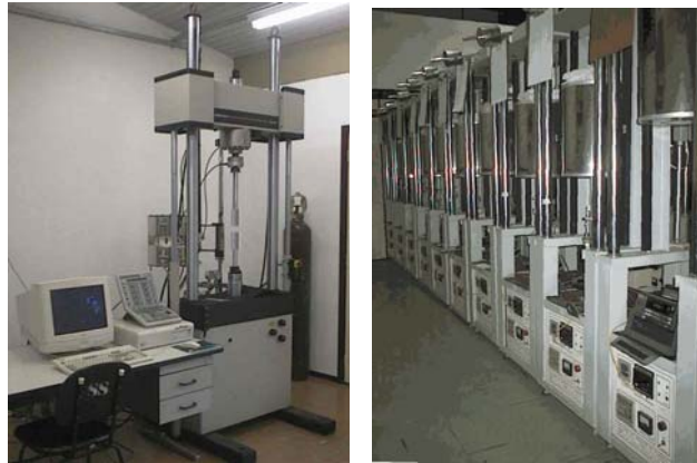
Figure 1 – Equipment used in this work: a) universal testing machine; b) Row of 10 constant stress/constant load creep machines.
