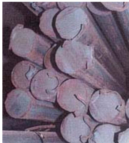
Figure 2: Bar ends cut with friction saw.
