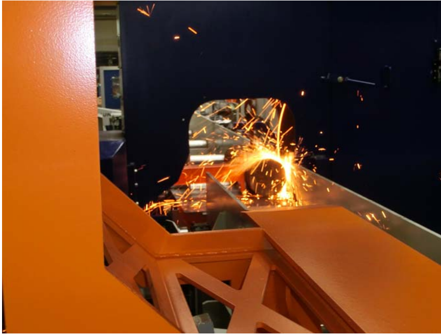
Figure 17: In-house functional testing of a cut-off machine prior to shipment.
