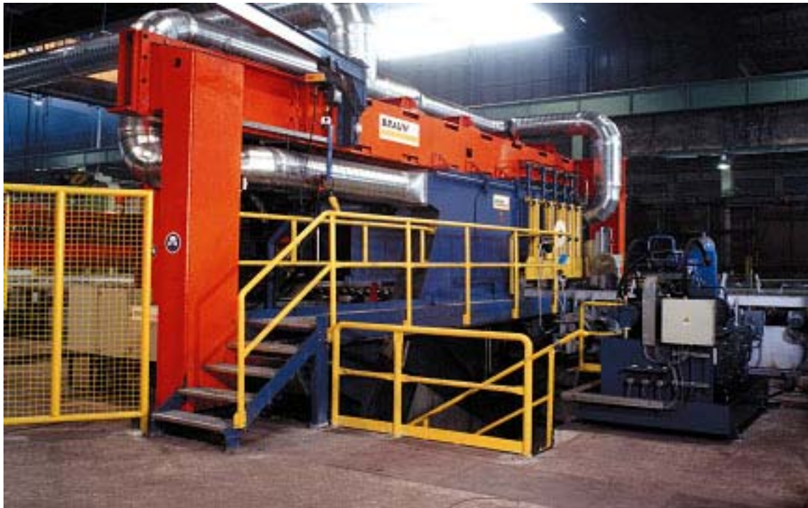
Figure 13: Braun gantry-type traverse abrasive cut-off machine, type TS 12 FP (for max. 1270 mm cutting wheel diameter, cutting width up to 2 300 mm) for hot cutting of plates and sheets as well as cold cutting of slabs (BÖHLER Bleche, Mürzzuschlag-Hönigsberg/Austria).
