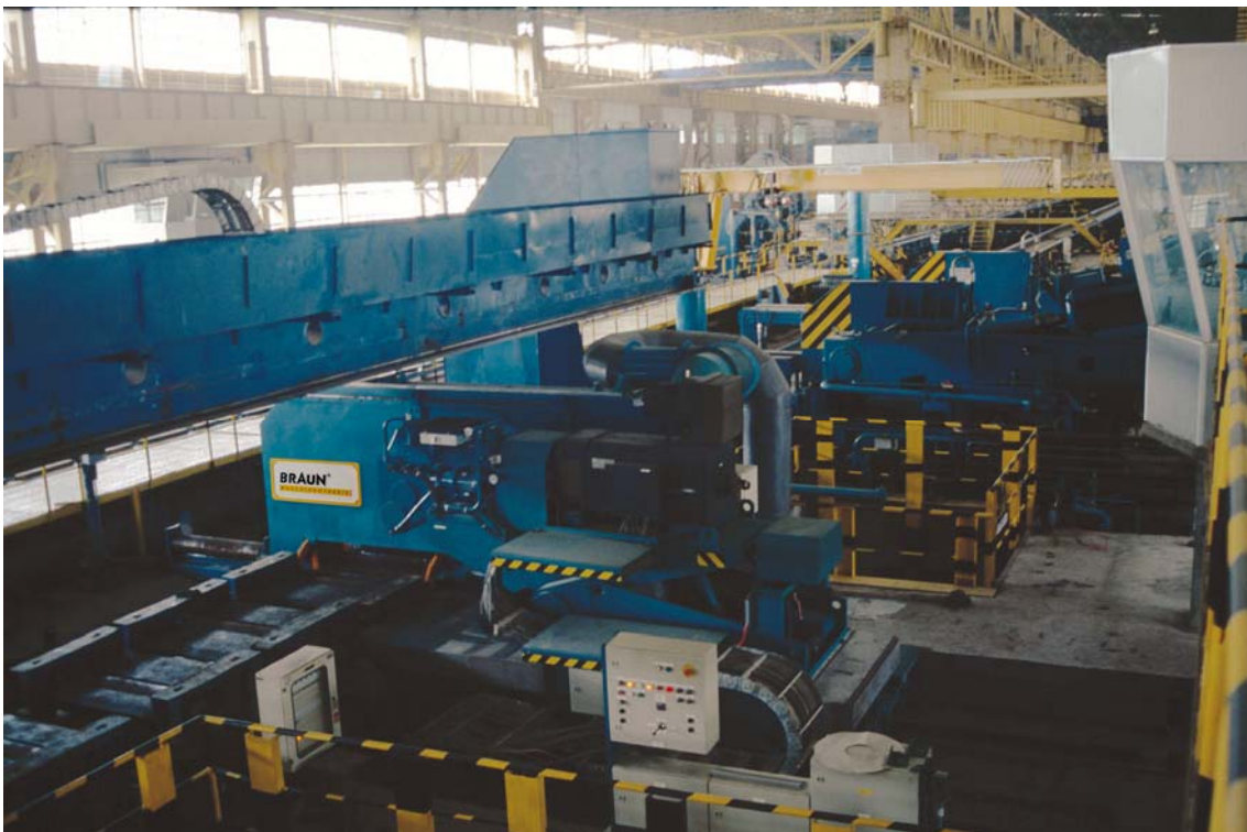
Figure 11: Braun traverse cut-off machine, type TS 12 F (for max. 1 270 mm cutting wheel diameter, cutting width up to 1 250 mm), for warm cutting of bars in layers (Jiangyin Cheng Special Steels, Jiangyin City, China).
