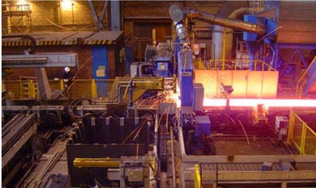
Figure 9: Braun abrasive cut-off machine, type TS 16 W (for 1 600 mm cutting wheel diameter), for hot cutting of blooms in primary mill (TATA Engineering Steels, Rotherham, UK).
