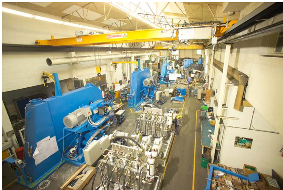
Figure 16: Pre-assembly of cut-off machines at BRAUN prior to shipment.
