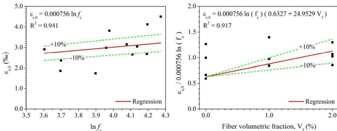
Figure 2. Regressions to define equation to estimate the peak strain.
