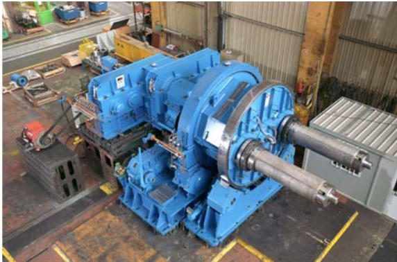
Fig.6 - Carousel Reel tested in Montbrison workshop
